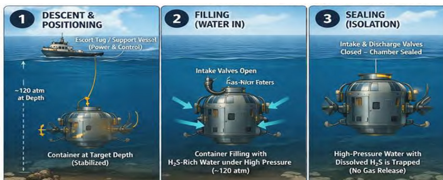
Figure 1: Overview of the buoyancy-controlled, towable subsea extraction system.
