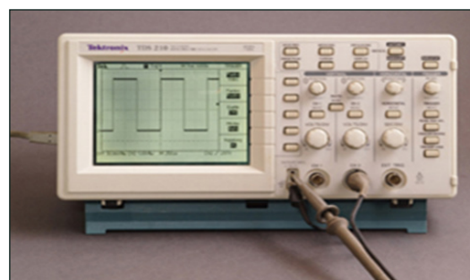
Figure 19: Encoder signals recorded on the oscilloscope
