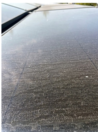
Figure 10: Bird Guano Rain Streaks on PV Panels.
