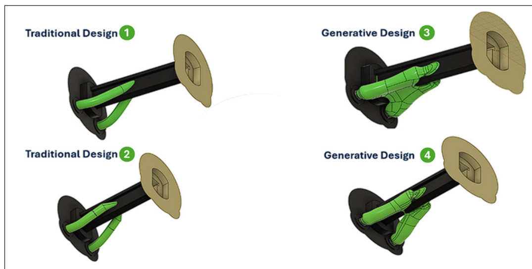
Figure 8: Four Alternative Design Solutions for the Air-Tube Interface
