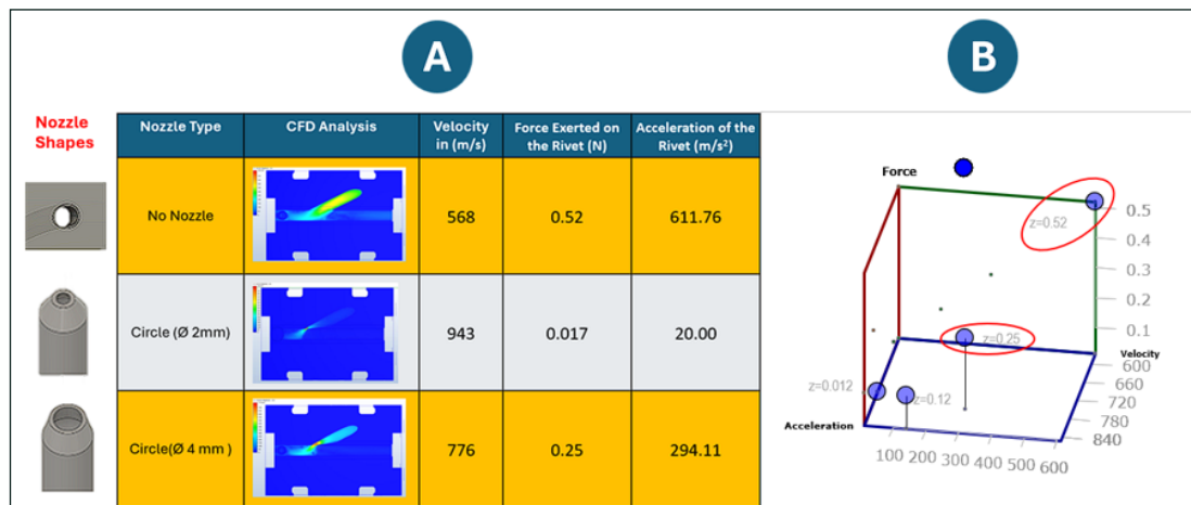
Figure 7-A: Alternative Design of Nozzles with CFD Simulation. Figure 7-B - Trade-off Curves of different Nozzle Shapes
