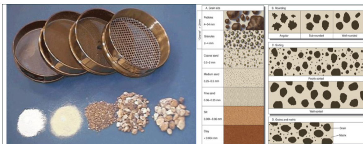
Figure 14: Grain Sizes Based on Cuttings Analysis From the Well Drilled in the Grgan Field
